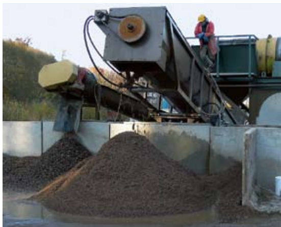
Cleaned and recycled gravel and sand, from remediation of soil contaminated with mercury and dioxin.
