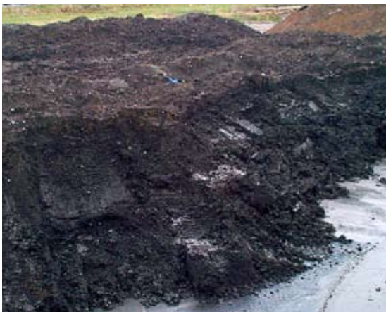
Soil and clay contaminated with PAH and lead demands many different treatment steps.
