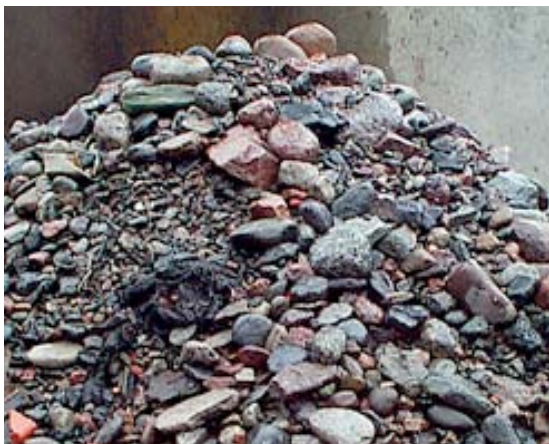
Cleaned and recycled gravel and sand, from remediation of soil contaminated with mercury and dioxin.
