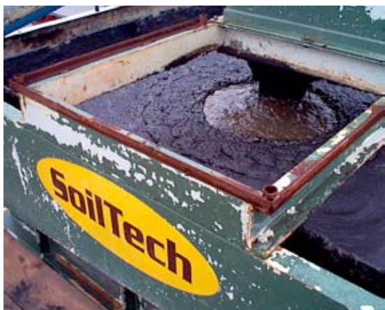
Oil sludge from oil-contaminated soil is separated through several steps including spillways.
